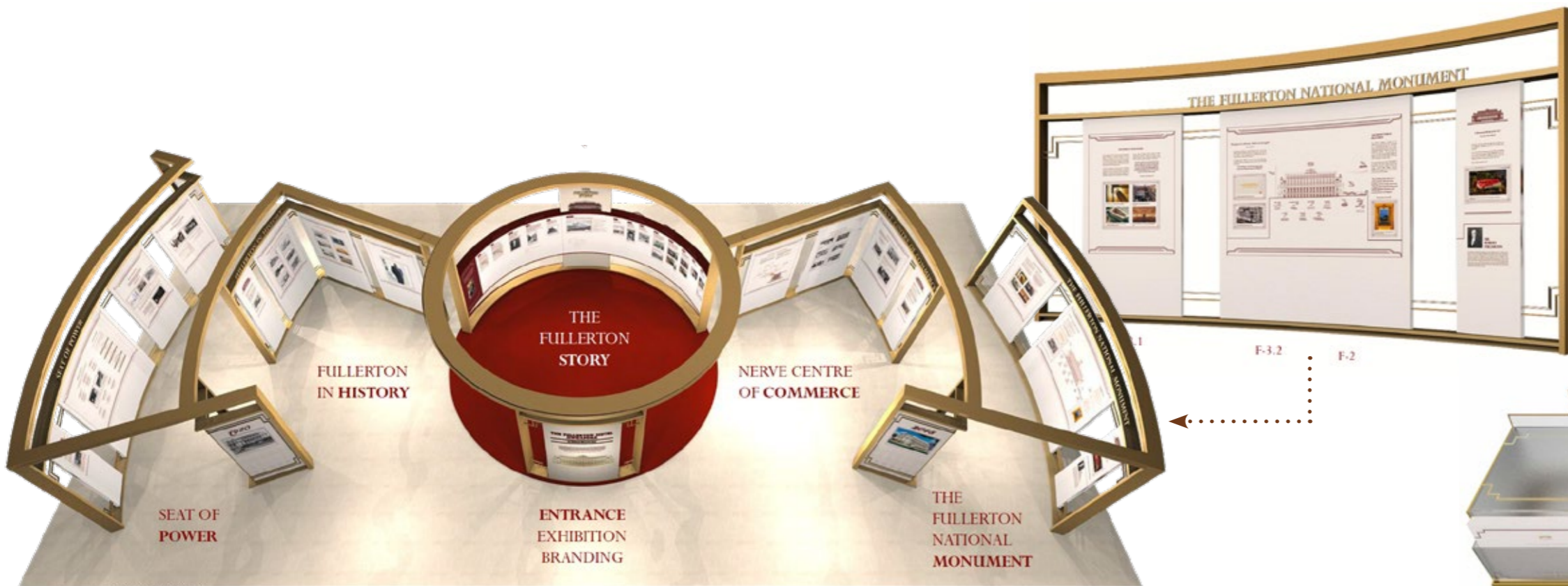
Design Overview | Continuous lighting pelmet holds the structure together, offers stability and allows for fast overnight setup
